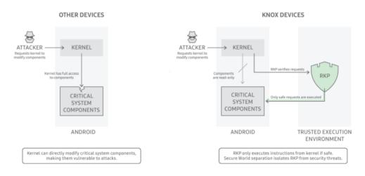
RKP's isolation from the kernel shrinks the Trusted Computing Base (TCB) and helps secure it from attacks designed to compromise the kernel. This unique ability enables RKP to detect and prevent the most common kernel attacks. RKP protections are grouped into three areas:
