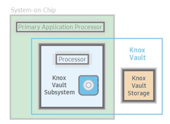
As a core component of the Knox security platform, Knox Vault is an isolated, tamper-proof, secure processor with its own core and memory, as well as an interface to dedicated, non-volatile secure storage. Knox Vault can:
