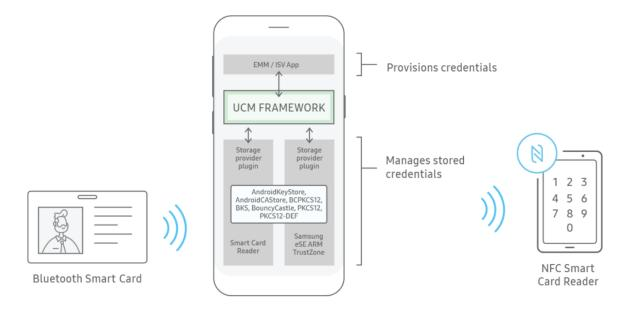
The Universal Credential Management (UCM) framework enables Android apps to access all credential storage devices through the same standard programming interface—the Java Cryptography Extensions (JCE) API via either:
