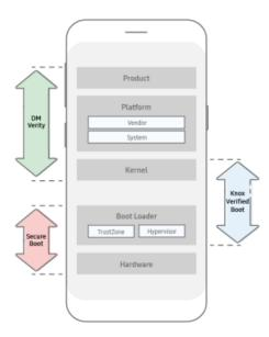
With KVB, component checks are conducted in the bootloader, and validations are made before system services are even started.
